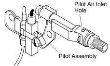
Figure 21 - Pilot Inlet Air Hole
